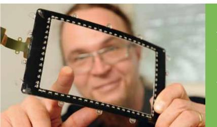
TactoTek combines familiar FTIR technology with VTT's printed electronics manufacturing method for the design and manufacture of touch panels for consumer electronics.
